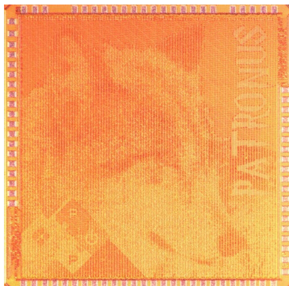
Fig. 2: Color picture of the PATRONUS chip taken through a Leica microscope
