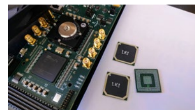
Fig.2: Packaged Loki chips and BaseJump motherboard (FPGA and BGA socket)
