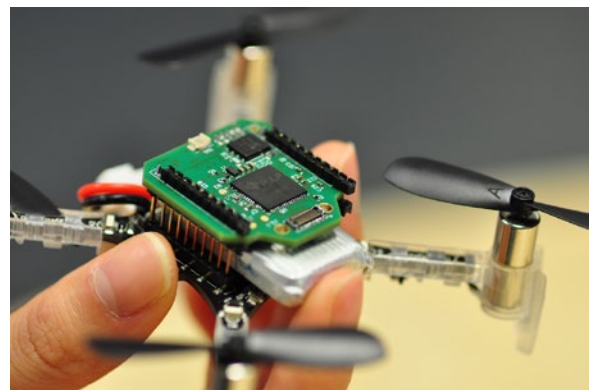
Fig.4: Mr. Wolf mounted on a nano drone. The chip is used to run a neural network to detect obstacles in real time
