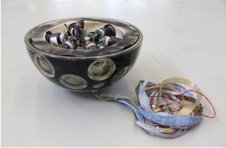
The RM5-hemisphere from the KM3Net project (Propriety KM3NeT Consortium).
