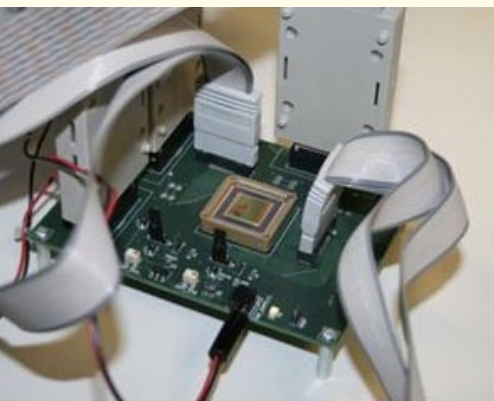
Fig. 2: Photograph of the test PCB with the packaged ASIC
