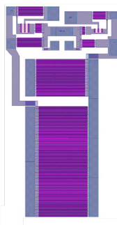
Monolithic integration of half-bridge and gate driver on imec's GaN IC platform.
