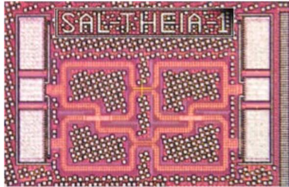
Fig. 1: Microphotograph of the test structure used to verify the D-band differential power combiner.
