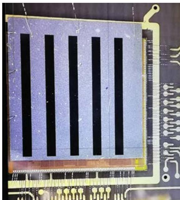
Fig.2: ASIC bump bonded onto a sensor
