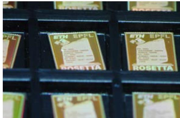
Fig.1: Rosetta dies in a waffle pack.
