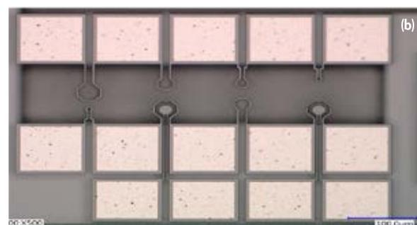
Fig. 2: Top-view die micrographs of (a) a variant of the comb drive actuator and (b) the piezo-resistive MEMS actuators.
