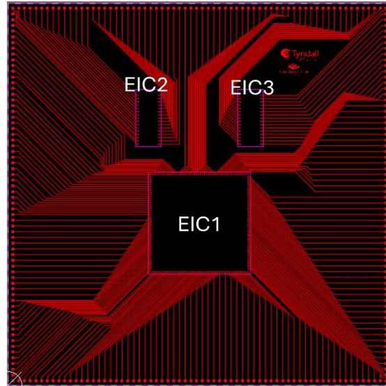
Figure 8. Tyndall designed/fabricated silicon interposer (30mm × 30mm) with given ICs dimensions. The interposer dimension is fixed and standard. The IC dimensions and number of DC connections can be changed, as needed.
