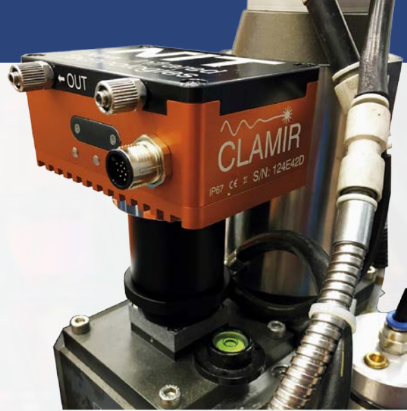
NIT’s high-speed IR sensor, CLAMIR, attached to a laser head for monitoring and controlling industrial additive manufacturing processes in real time.
