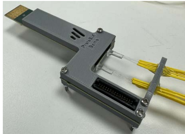
Fig2: 56Gbs silicon photonic transceiver system for space communications.
