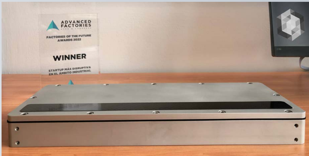
Fig.1: The PhotonAi® camera contains hybridised sensors for multi-channel photon counting during line scan inspection.
