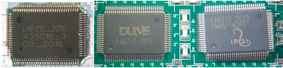
Fig2: LARZIC chip in a 100 pin PQFP 0.65mm pitch package for low-volume production in 2016, 2020, and 2023.
