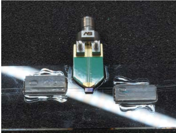
Fig.4: Sample for irradiation experiments on ring modulators.
