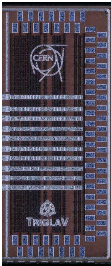
Fig.1: Microscope image of TriglaV with a 1mm x 2mm silicon area.
